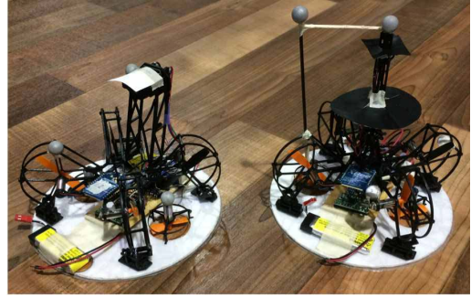
Fig. 2. Left: autonomous pursuer hovercraft with onboard camera. Right: target hovercraft with IR light tower.
