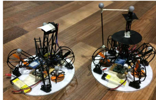
Fig. 1. Autonomous pursuer hovercraft with onboard camera (left), and target hovercraft with IR light tower (right).
